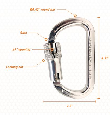
The Aluminum Carabiner with 3/4" gate is specially designed to be both high-strength and easy to use. Its gate is certified to withstand loads up to 3,600 lbs, is self-closing and self-locking, and can be opened with just one hand. All aluminum carabiners compliant with the most current ANSI and OSHA regulations.
