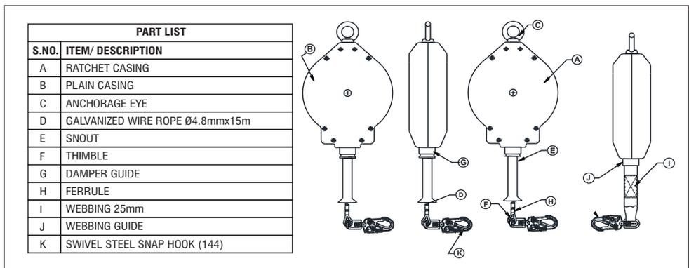
**ARRESTA Self Retracting Lifeline:** Includes a swivel eye anchorage, self-locking swivel snap hook with impact indicator, and 3/16" galvanized wire cable/1" Polyester Webbing. SRL also comes with a Karabiners and tag line to be used with the device to avoid improper use.
