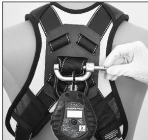
Slide Connector through loosened web straps placed below the D-ring, then pull straps tight.
