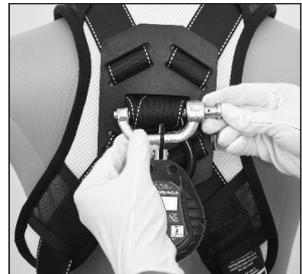
Push the pin inside the grooves of the connector to ensure locking.
