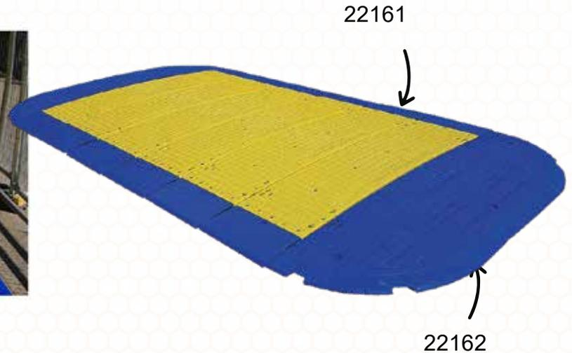
The Fiberglass Road Plate is a modular system of singular linking units. HS20-44 rated, this road plate is suitable for 97,000 lb vehicles over a 18" wide trench.
